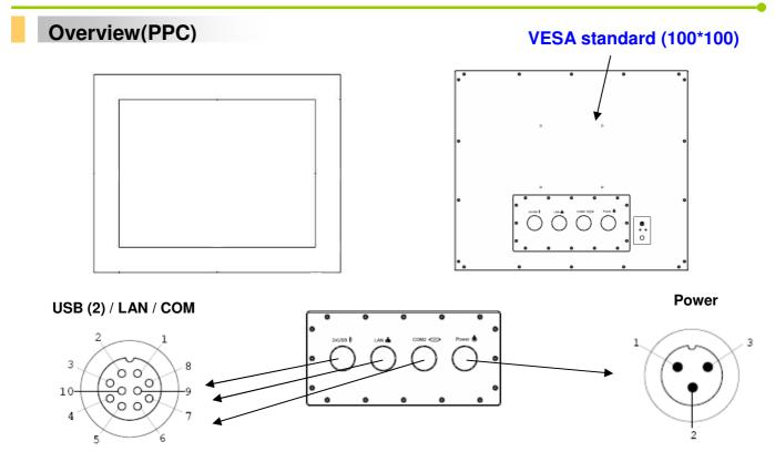
Full IP65 PPC provides Four IO. One is 2 x USB(10 pin) in the left side, LAN and COM connecter in the middle, power connecter in the right side. All of the connectors are IP65 level and fool-proofing design, it helps the end user to installation USB, LAN and COM cables correctly.
