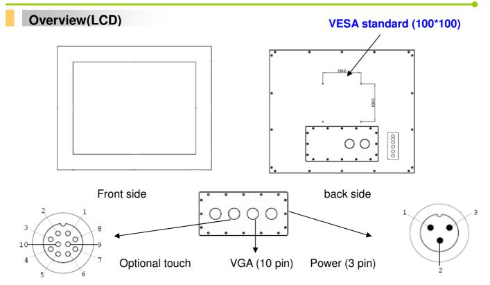
Full IP65 MONITOR provides two IO in back side. One is power (3 pin) in the right side, anthers are VGA and optional touch interface (USB or RS232) in the left side. All connectors are IP65 level and fool-proofing design; it helps the end user to install correctly.
