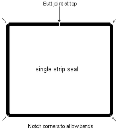
*Note: The strip can touch the reflector stripes if absolutely necessary, but by no more than 1 mm. If more than 1 mm contact is necessary, a hard bezel material such as ABS plastic can be used instead of strip, but this will not make a splash-proof seal. Firm contact with the touch screen glass is required as a minimum dust seal.*
