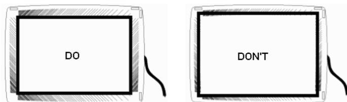
2. The seal must be fully compressed all the way around. This provides a splash-proof seal which will not allow liquids to wick behind the seal. It also creates a stable signal, even if a user presses hard on the bezel.
