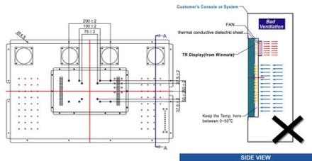
**⚠ MAKE SURE HAVE THERMAL SOLUTION ON YOUR CONSOLE OR SYSTEM, OR IT WILL CAUSE THE DISPLAY SHUT DOWN.**
